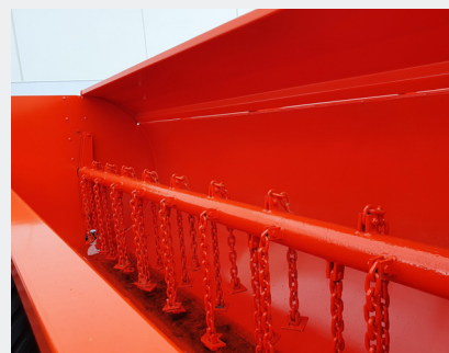
Heavy duty rotor with chains and flails
