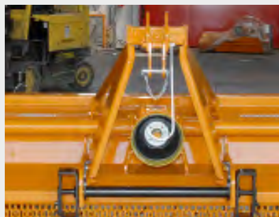
Heavy duty floating/fixed headstock
