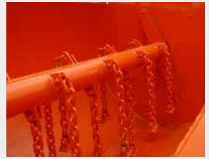
Heavy duty rotor with chains and flails
