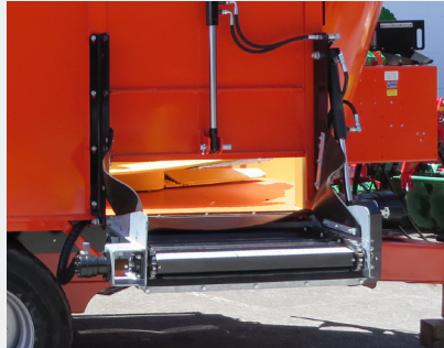
1m wide feed door for even feeding
