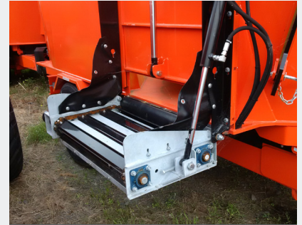
Slat and chain elevator, low maintenance
