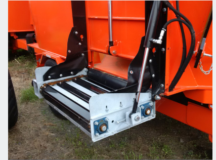
Slat and chain elevator, low maintenance
