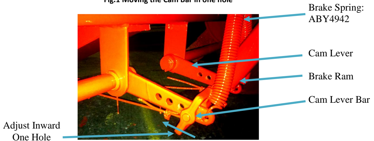
Fig.1 Moving the Cam Bar in one hole
