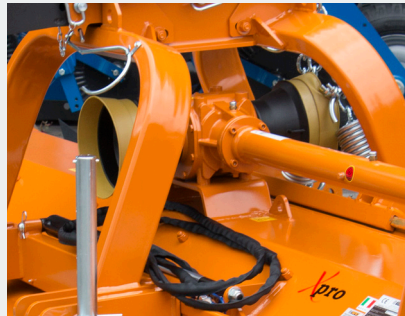
Heavy duty gearbox with through shaft and double free wheel
