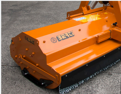
Double skin chassis made of Strenx
