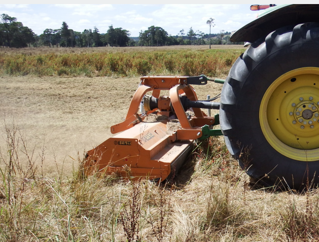
Double skin chassis made of Strenx
