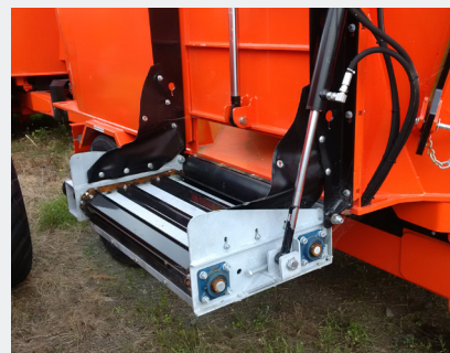
Slat and chain elevator, low maintenance
