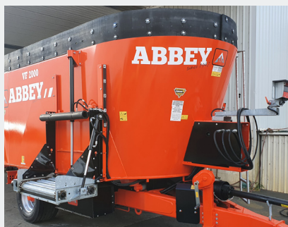
Independent chassis to allow for large torque loading
