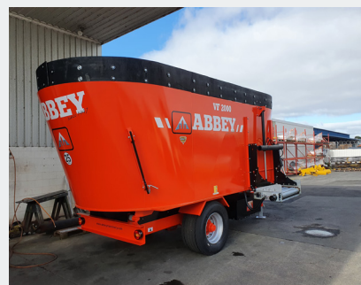
Rolled walls for superior mixing
