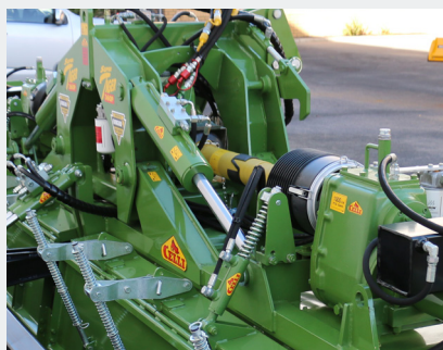
Hydraulic folding with safety locks
